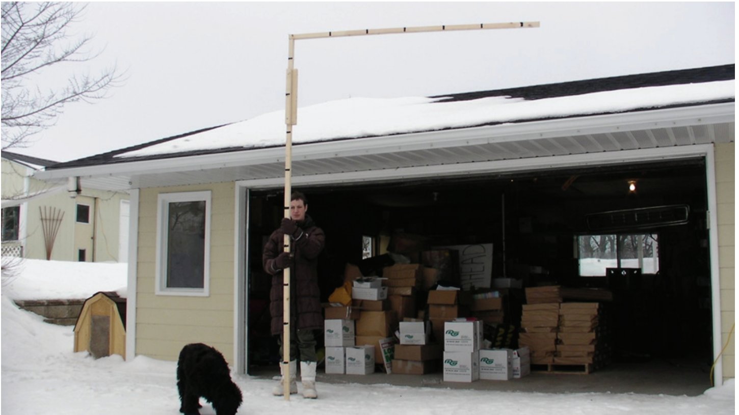
Photo showing measuring apparatus for maximum MUTCD height and distance standards for speed-limit signage (maximum 3.0 meters high by maximum 2.0 meters distance (reach) from the curb)
